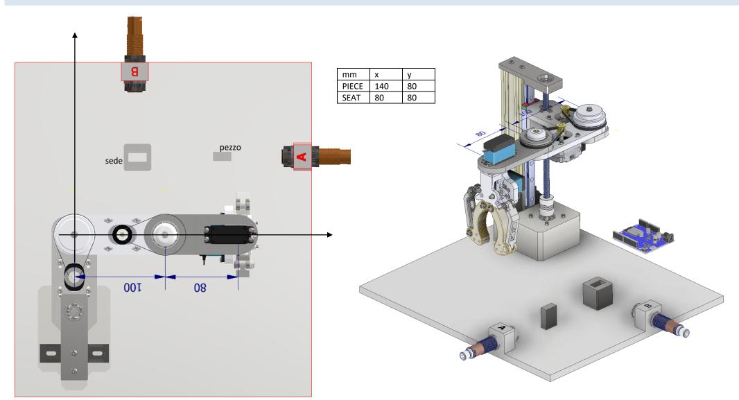
When the ultrasonic sensor "A" detects the presence of a "piece", the robot, from the default position, positions itself on the piece, picks it up and deposits it in the "seat" only if the ultrasonic sensor "B" detects the presence of the seat. If the seat is not present, an emergency flashing light L (12V – 200mA) must be activated. After calculating the angles with inverse kinematics draw the electric circuit and write the Arduino code.
